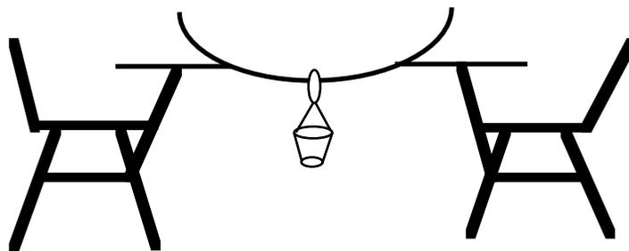
**Collecting Data:** Find the breaking weight for pieces of pasta that span gaps of different lengths – from 2 - 6 inches. Then try thicker “bridges” by using 2, 3, 4, and 5 strands of pasta. Record the (length, strands, weight) data in a table like this.
